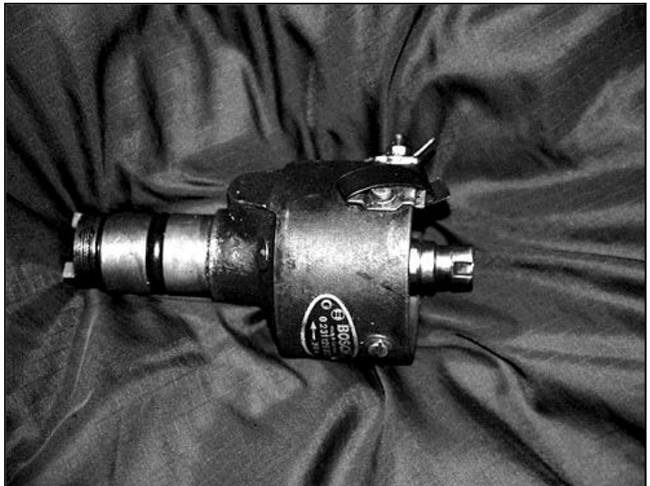
The .010 Bosch Distributor eliminated the vacuum advance system and is very similar to the .009.
